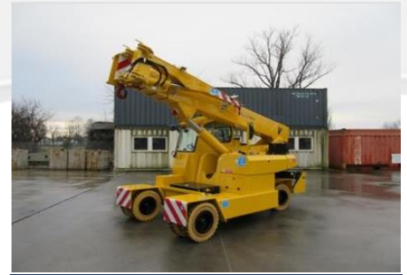
Hydraulic jib that can be turned on the boom side when not used
